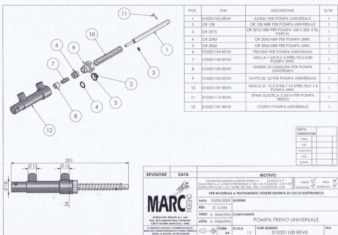
Introduction: the master brake cylinder replacement set, must be installed after having bled the hydraulic system. Also before the installation all the O-rings must be greased for a clipping free fixing.
