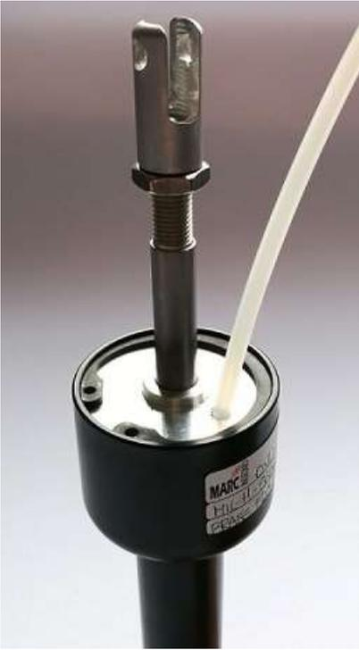
The other end of this flexible hose is inserted into the bleeder reservoir so that allows the oil in the aircraft tank to overflow and enter in the bleeder reservoir.
