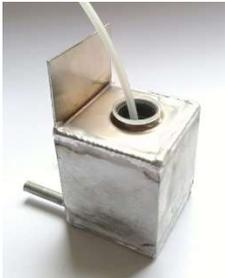
The end of the hose is inserted into the bleeder reservoir to allow the oil in the aircraft tank to overflow and enter the bleeder reservoir.
