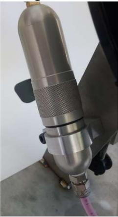
Connect the output of the electric bleeder to the filling valve of the brake caliper system.
